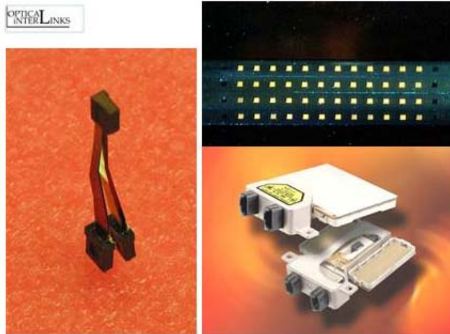
Fig 18: Stacked Waveguide Array Interface Coupling: A four by twelve stacked waveguide array with 125 micron center to center spacing vertically and horizontally is shown. The array is created from 4 waveguide films with imaged guides creating the 90 degree bend in the 4 film array on the left. Each of the 4 waveguide array films contains 12 precisely located operating waveguides. Two films are stacked and connected to a 12 over 12 MT connector ferrule with spacing optimum for the same 12 over 12 fiber coupling. The guides were within +/- 5 micron centering individually and with run out. The final package with the wishbone shaped waveguide assembly to interface to the components were all developed and beta tested by Teraconnect for high data rate transceiver before market conditions terminated the effort.
