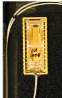
Fig. 25: Novel Waveguide Designs for an 8 to 1 Combiner An 8 to 1 combiner was created using small width input waveguides with optimized waveguide designs. The unique design combines all inputs with good coupling and low excess loss of around ~2 dB coupling into a single optical fiber. OptiComp Corporation installed multi-wavelength combiner on their board transmitter unit shown in the figure. The waveguide design also operates as a splitter with ~1dB excess loss for the receiver side of the circuit.
