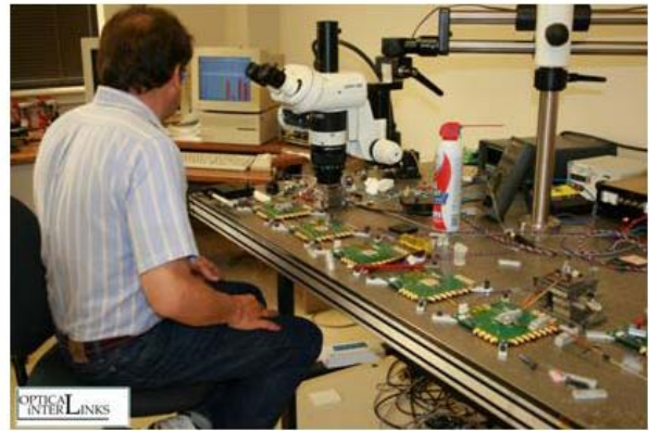
Fig. 28: Pilot Manufacturing Assembly Scale up for assembling TxRx parts has begun to increase production and reduce costs with staged workstations for the waveguide lens to substrate transmitter and receiver described in figures 11 thru 13.
