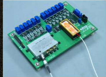
Fig. 25: Novel Waveguide Designs for an 8 to 1 Combiner An 8 to 1 combiner was created using small width input waveguides with optimized waveguide designs. The unique design combines all inputs with good coupling and low excess loss of around ~2 dB coupling into a single optical fiber. OptiComp Corporation installed multi-wavelength combiner on their board transmitter unit shown in the figure. The waveguide design also operates as a splitter with ~1dB excess loss for the receiver side of the circuit.
